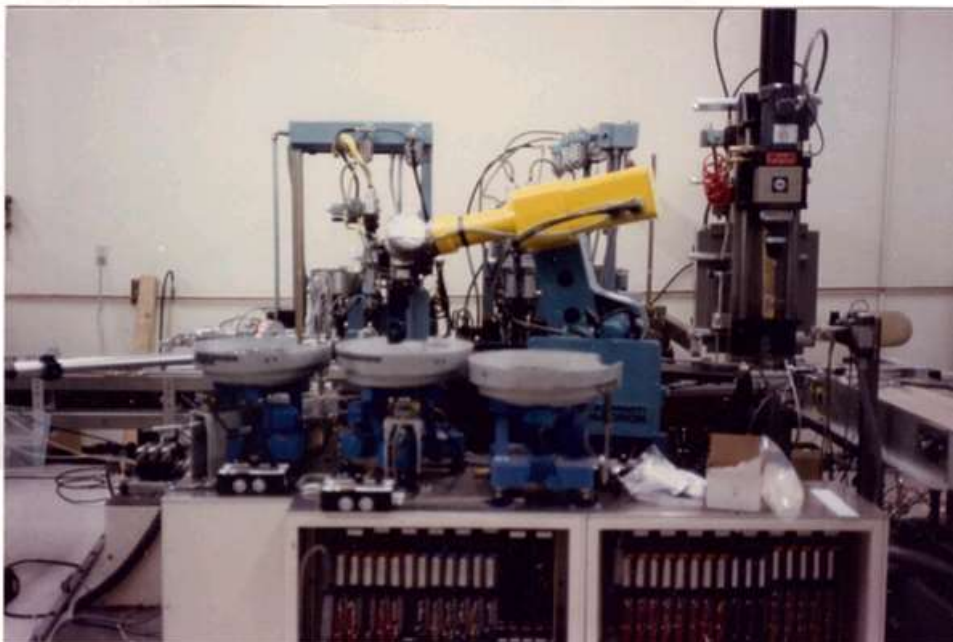
Higher production levels and more consistent product quality are achieved by Shugart with this floppy disk drive assembly workcell.
