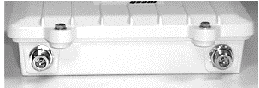
Top: 2 N-Female connectors to Antennas
