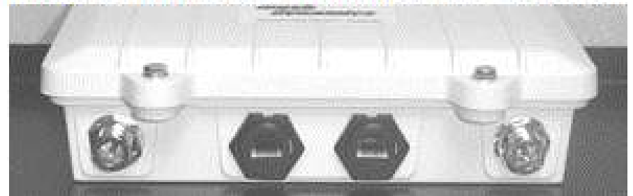
Bottom: 2 N-Female, 2 Ethernet Ports with POE
