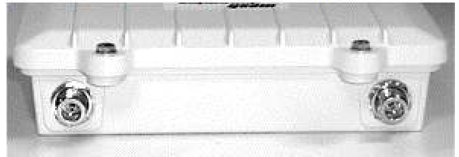
Top: 2 N-Female connectors to Antennas
