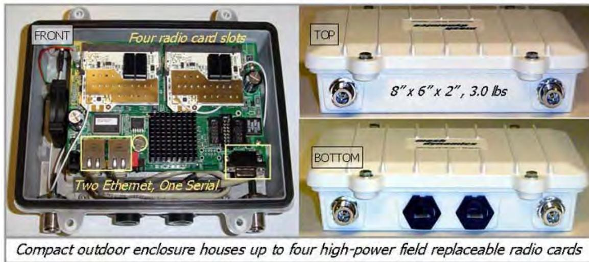
*Compact outdoor enclosure houses up to four high-power field replaceable radio cards*
